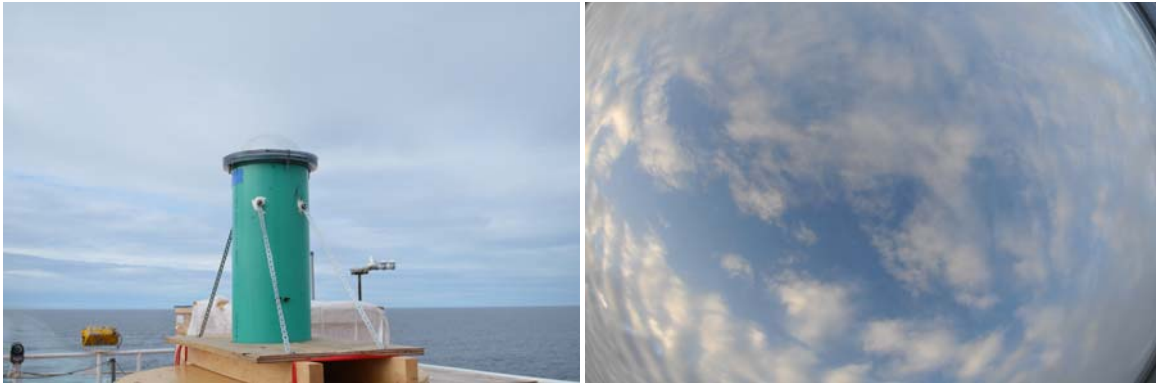
Figure 7. All Sky Camera mount and sample image
