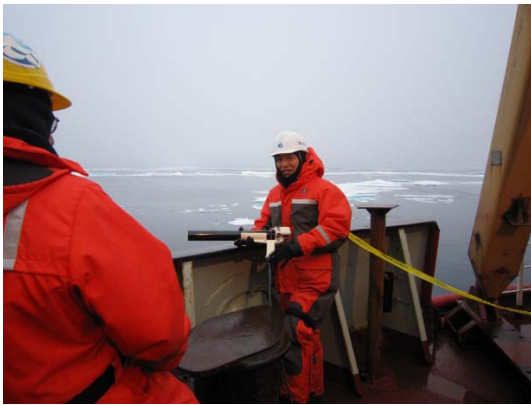
Figure 1: XCTD probe deployment from the ship's stern (2011) and XCTD data converter MK-150.
