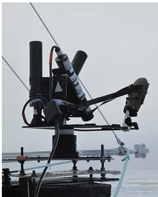
Figure 8. Bow mounted HyperSAS instrument with time lapse camera and a CNR-1 net radiometer (Alice Orlich) in the background.
