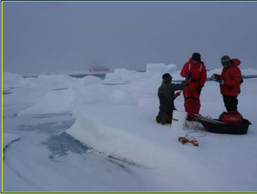
Photo 4. Volunteers persist along a 150m drill transect line with the 2" auger system and CTD.
