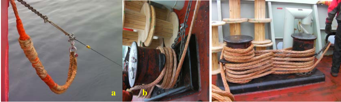
Figure 4. The photographs of dragging line. (a) connection part of weak link, 1995m wire, chain, and ship's berthing line. (b & c) the chain and berthing line lashed to bitt on the fore deck.
