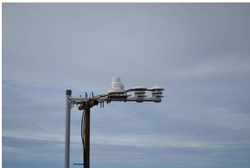
Figure 2. Radiation sensors mounted on the port side, including the UV sensor, pyranometer and pyrgeometer.
