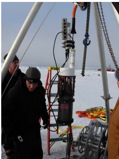
Figure 1: SAMI being deployed on ITP 65 during the first ice station. A conductivity and dissolved oxygen sensor are also deployed as part of this system.
