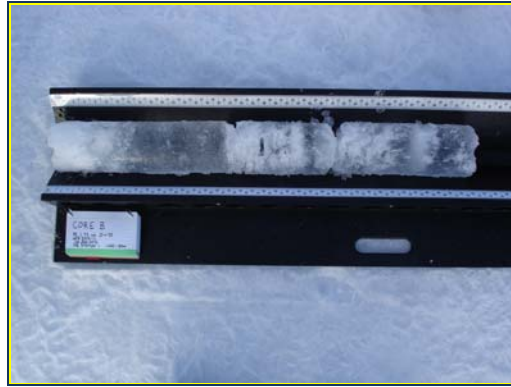
Photo 5. A core section is measured for length before temperatures are taken and the core is sectioned into 10cm pieces for later analysis.
