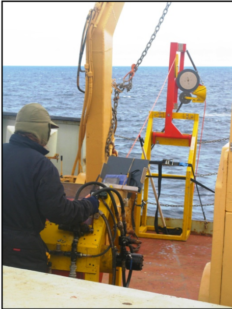
Figure 3: Hydraulic winch and line puller for deployment of the VMP500 through the A-frame doors.
