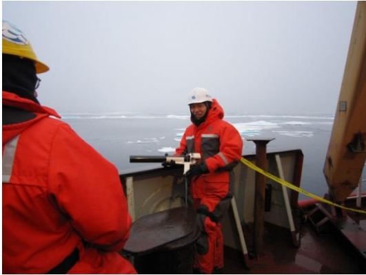
Figure 1: XCTD probe deployment from the ship's stern (2011) and XCTD data converter MK-150.
