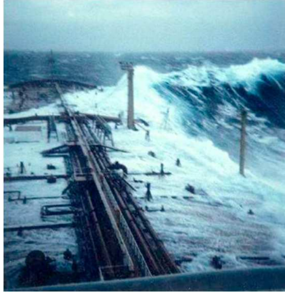
Figure 8: Rogue wave breaking over a supertanker in a storm off Durban, S.A. in 1980. The mast seen starboard stands 25 m above the mean sea level. The mean wave height at the time was 5-10 m. Photo: Phillipe Lijour, first mate.
