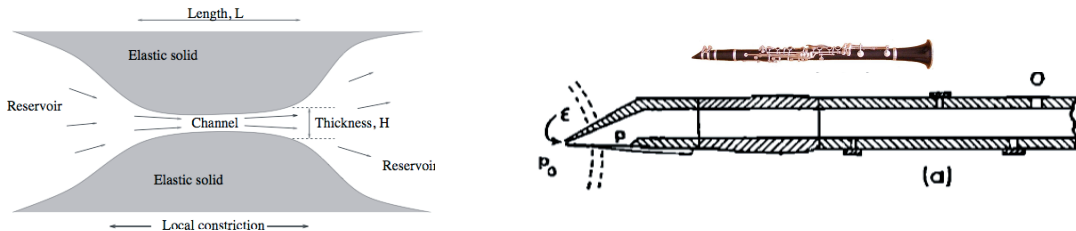
Figure 1: Oscillating reed in a clarinet (Backus 1963 [1]) or rock exciting and interacting with standing waves in the adjacent reservoir [5].
