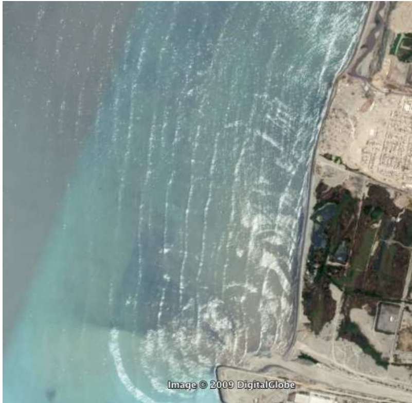
Figure 1: Waves approaching the coast of Callao (Peru). It is possible to see that as the waves approach, their crests sharpen whereas their troughs flatten (Google Earth, around 12^{\circ}01' \text{ S} , 77^{\circ}09' \text{ W} ).
