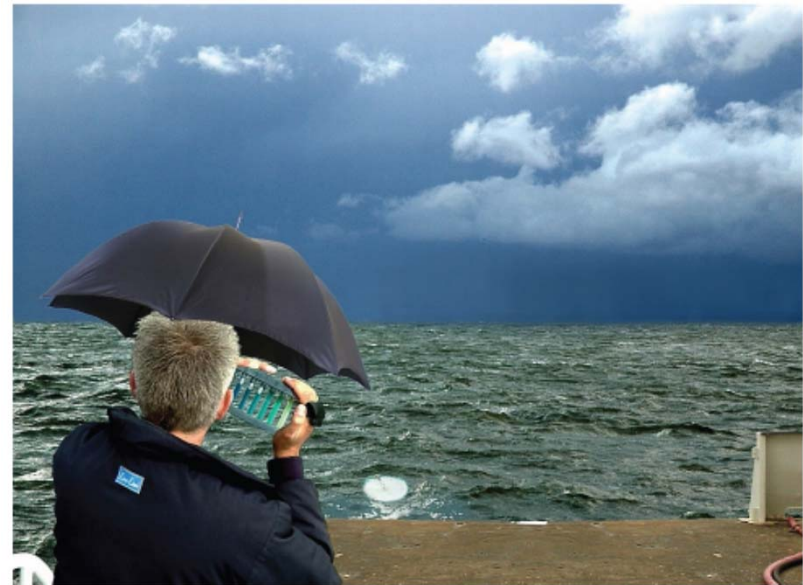
FIG. 4 A FU observation is taken, at the shady side of the vessel, above a submersed Secchi disc, with the disc lowered to a depth of approximately half the Secchi disc depth. The reading of the scale should be done in the shadow.
