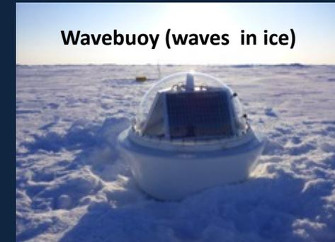
Wavebuoy (waves in ice)
