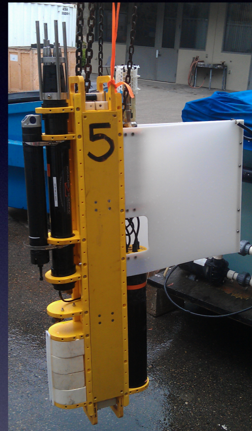
Wave-powered vertical profiler (SIO) Lucas/Pinkel chi J. Moum/J. Nash, OSU
