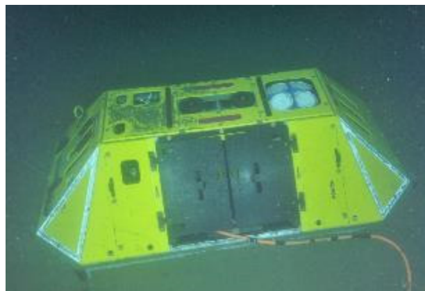
Benthic Experiment Package (ADCP visible on top), summer 2014.
