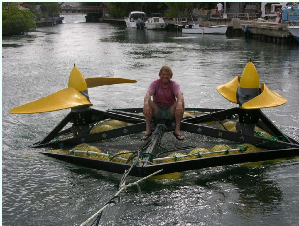
A pair of 98"-diameter, 5.44 kW Flygt thrusters for "twin-screw" operation
