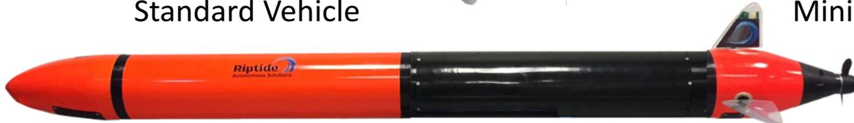
Standard Vehicle with flooded payload bay
