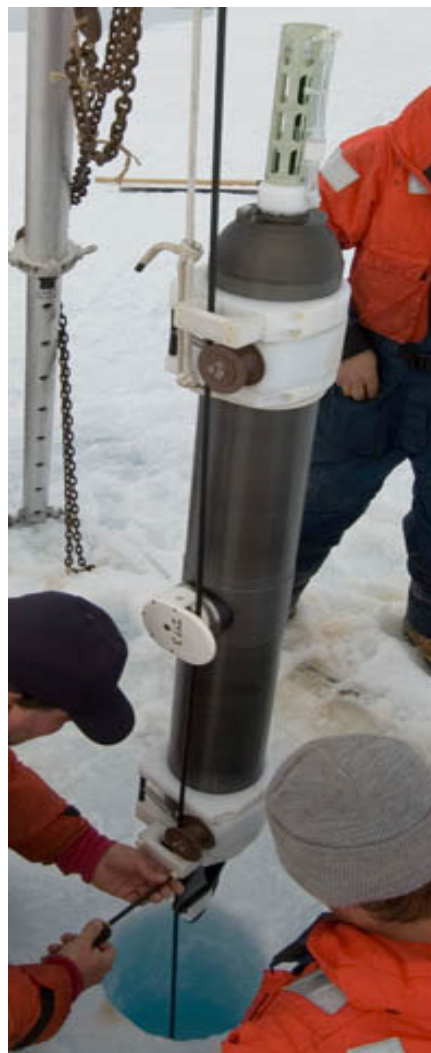
Figure 7: Attaching ITP to mooring wire during deployment.
