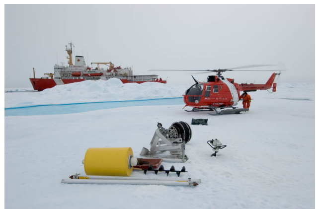
Figure 11: Transporting ITP gear to deployment sites using hand sleds and helicopters (in slings and cargo).
