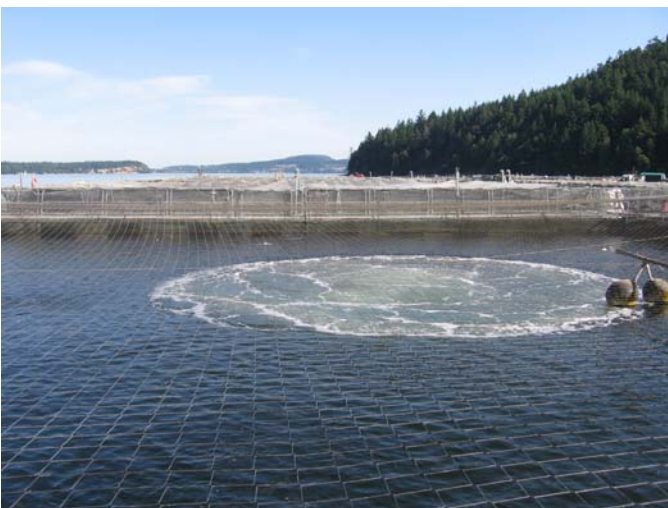
Figure 28. Upwelling water inside a pen a minute after a compressor and airlift assembly was turned on.
