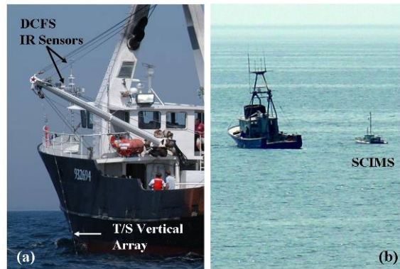
Figure 10. a) Instrumentation deployed on the Nobska during the 2003 IOP. Bow instrumentation included a direct covariance flux system and IR radiometers. The boom supported an array of temperature/salinity sensors for high-resolution vertical profiles. b) Photo taken from the Air-Sea Interaction Tower at MVCO of the SCIMS catamaran accompanied by R/V Asterias during a southeasterly survey transect on August 15, 2003. Numerous banded surface film features (light areas) evident in the field of view were quantified by SCIMS instrumentation.
