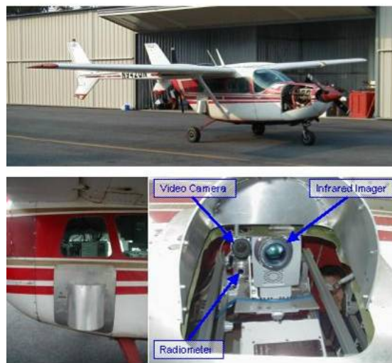
Figure 11. The top panel is a picture of Cessna Skymaster chartered for CBLAST-LOW 2002 and 2003. Picture on the bottom left is a close-up of the cargo door on the Cessna Skymaster that was modified to accommodate our downward-looking instruments. Picture on the bottom right is a close-up of the downward-looking infrared imager, collocated video camera, and collocated, narrow FOV infrared radiometer.
