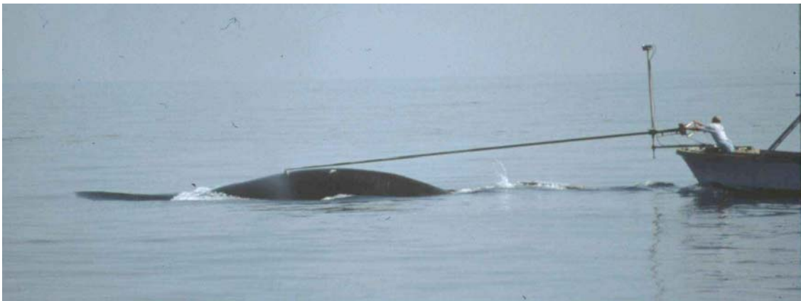
The cantilevered pole system laying an acoustic sounder on a right whale
