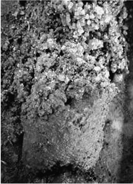
Fig. 3. Photograph of core sample showing transition from overlying sand to hard layer atop the weathered bedrock.
