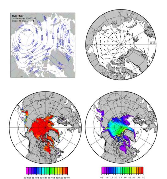
Validation of Polar Ice Prediction System (PIPS) 2.0 Ice Motion (top right) against IABP SLP and buoy motion (top left). The lower figures show the analyzed ice concentration (bottom left) and thickness (bottom right). Courtesy of Ruth Preller, NRL.
