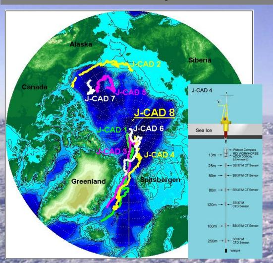
In the multiyear ice zone of the Arctic Ocean, ice-drifting buoy observation is the most useful method to monitor the oceanographic condition even under the severe environmental condition. However, ....
