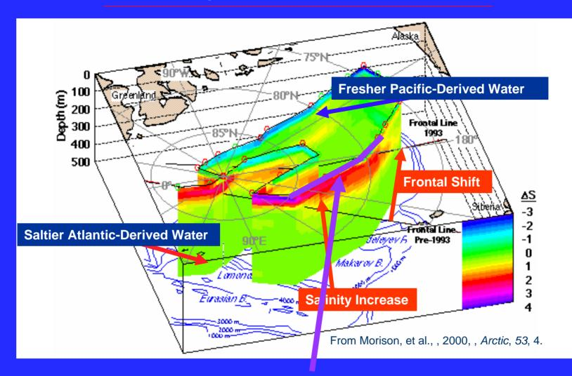
Section across the Makarov Basin gave the most profound indication of ocean change in the early 1990s. It is hard to make, especially with drifting buoys
