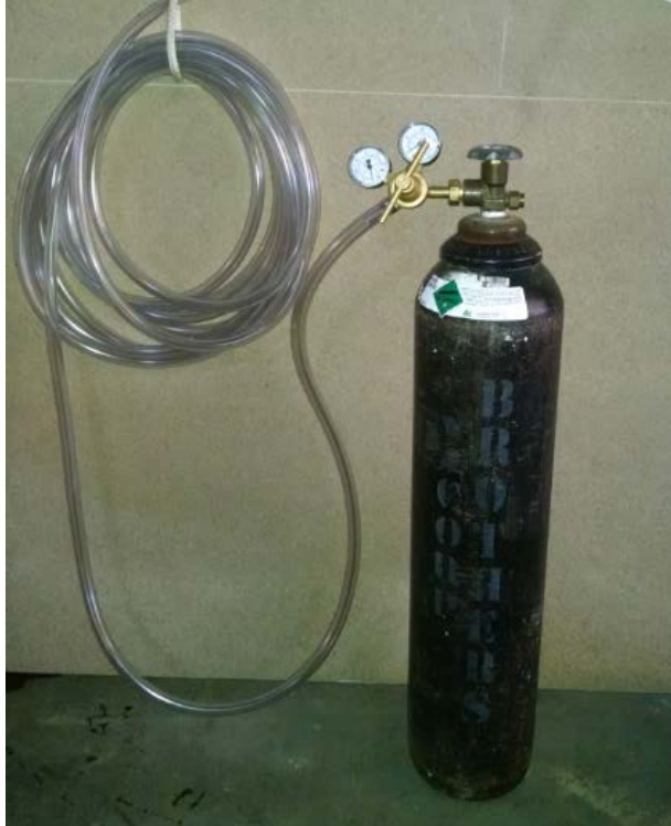
Figure 5: Nitrogen Tank, Regulator and Flexible Tubing
