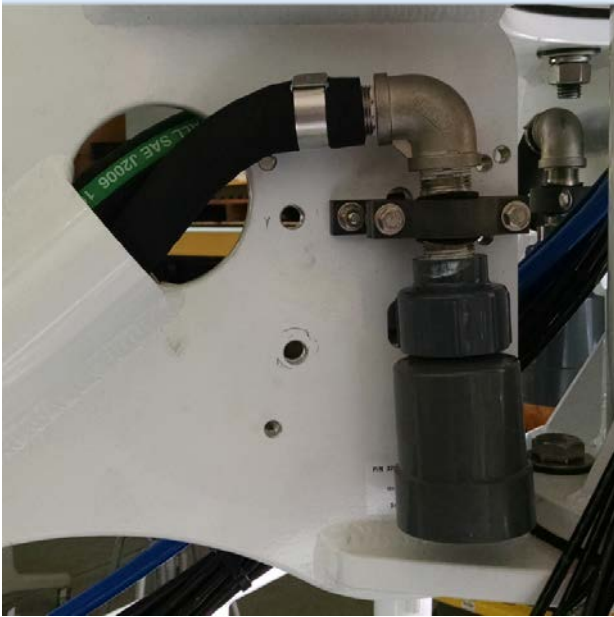
Figure 9: Vent Valve to be removed
