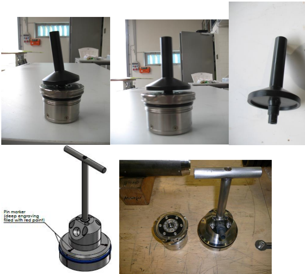
Figure 5. Protection cap (upper) left in the top of the borehole plugs. This will be removed before attaching the cap connector (lower)
