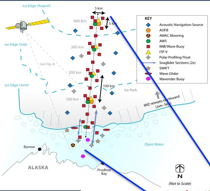
Ice-based array deployed by aircraft in April (full ice cover).
