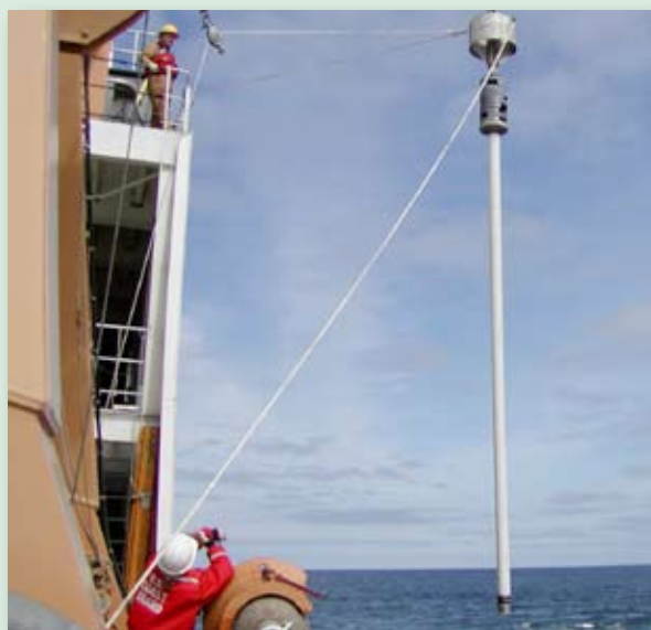
Large Diameter Gravity Core (5 meters long) being launched from USCG Icebreaker Healy in the Bering Sea, July 2002. Used to collect sediments from the seafloor that reveal the ancient history of Earth's oceans and climate.
