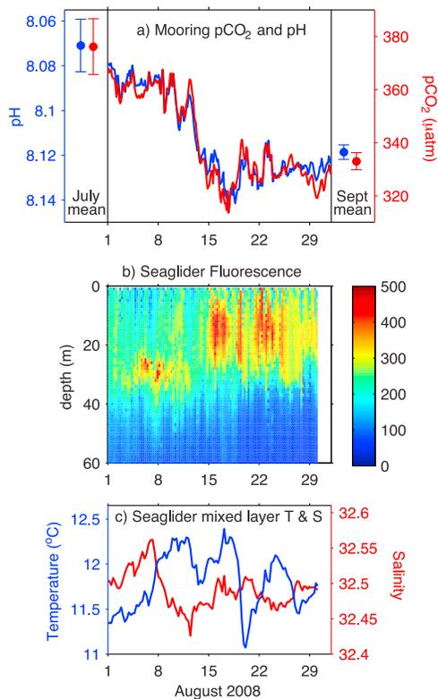
**Figure 2.** (a) Aqueous pCO<sub>2</sub> (red) and pH (blue) measured at the surface from a mooring at Station P. pH scale is reversed. Means and standard deviations for July and September 2008 shown. (b) Raw chlorophyll fluorescence signal measured by a Seaglider within 35 km of Station P. (c) Seaglider temperature and salinity averaged over upper 20 m.
