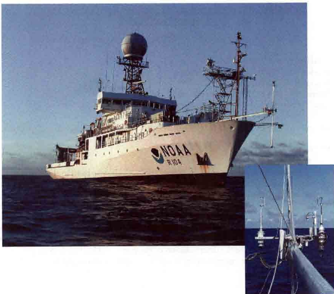
Figure 1: Images of the NOAA research vessel Ronald H. Brown with the bow boom/mast system used in GasEx-2001.
